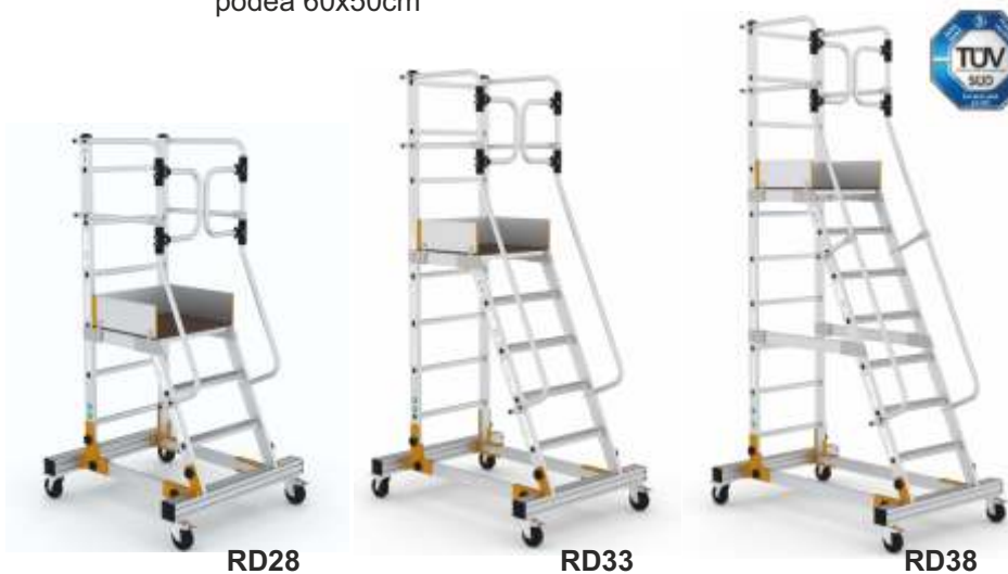
8697817585718 Platforma RD38 - Platforma mobila profesionala cu 7+1trepte, Hlucru=3,8m podea 60x50cm
